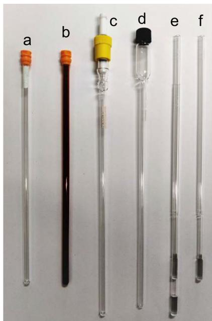
**Fig. 2.** A selection of 5 mm O.D. NMR tubes. (a) plain borosilicate, polyethylene cap; (b) amberised borosilicate; (c) J Young valve capped borosilicate; (d) titration tube with screw cap; (e) Shigemii tube with insert – sample held between two ‘matched’ solid glass plugs; (f) Shigemii insert.
